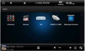
Control4 does it all, though. Since the HC-250 sits on the same home network as the rest of your 'net-connected devices, it remains in constant communication with those devices and sends two-way control commands via WiFi or Ethernet. That includes satellite receivers from the most popular service providers, TiVo and other cable DVRs, TVs and AV receivers from a number of manufacturers, as well as popular media streamers.
